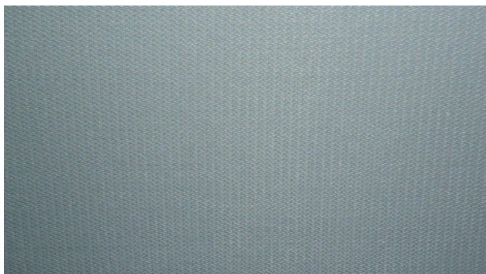
FM Fire Duct systems use a glass fibre cloth, bonded directly on to steel ductwork to give fire resistance of up to four hours.
